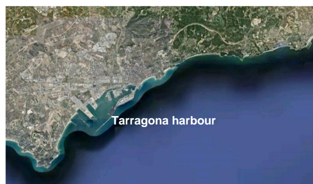
Fig. 13. Plan of the Tarragona Port and surrounding coast, showing that headlands prevent waves from NE and SW from reaching the port area.
