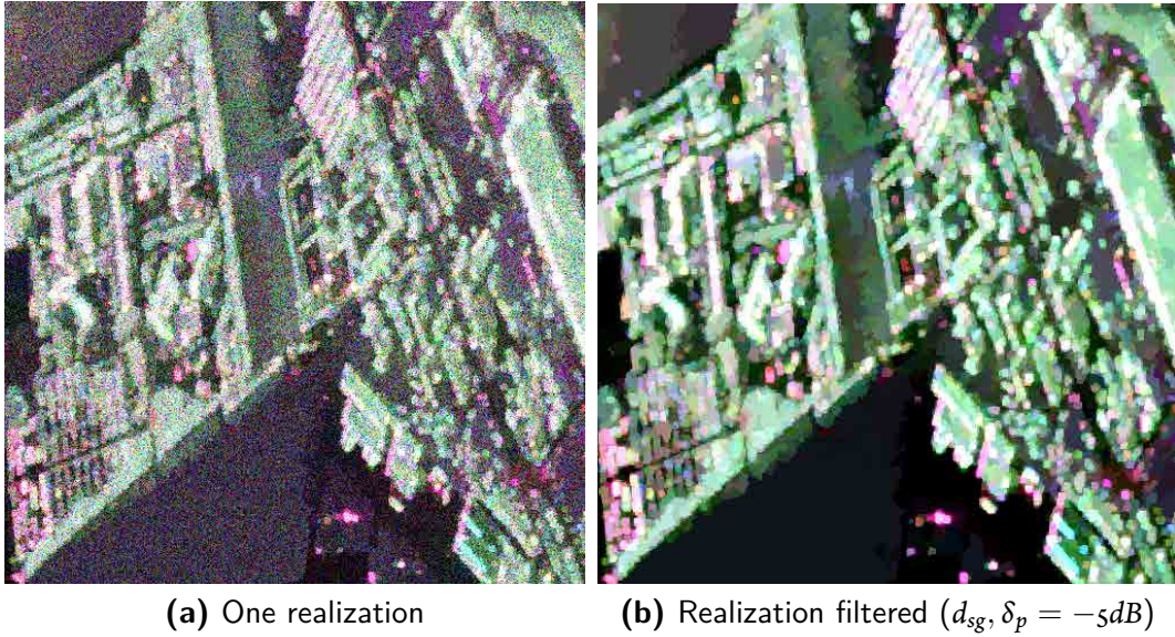
Figure 4.27: One realization of the urban simulated ground truth and the corresponding filtered image ( |S_{hh} + S_{vv}| , |S_{hv} + S_{vh}| , |S_{hh} - S_{vv}| ).
