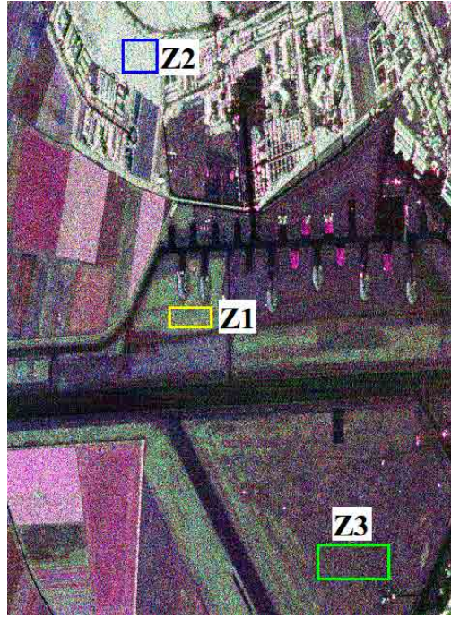
Figure 4.17: Homogeneous zones manually selected over the original image for the quantitative analysis ( |S_{hh} + S_{vv}| , |S_{hv} + S_{vh}| , |S_{hh} - S_{vv}| ).
