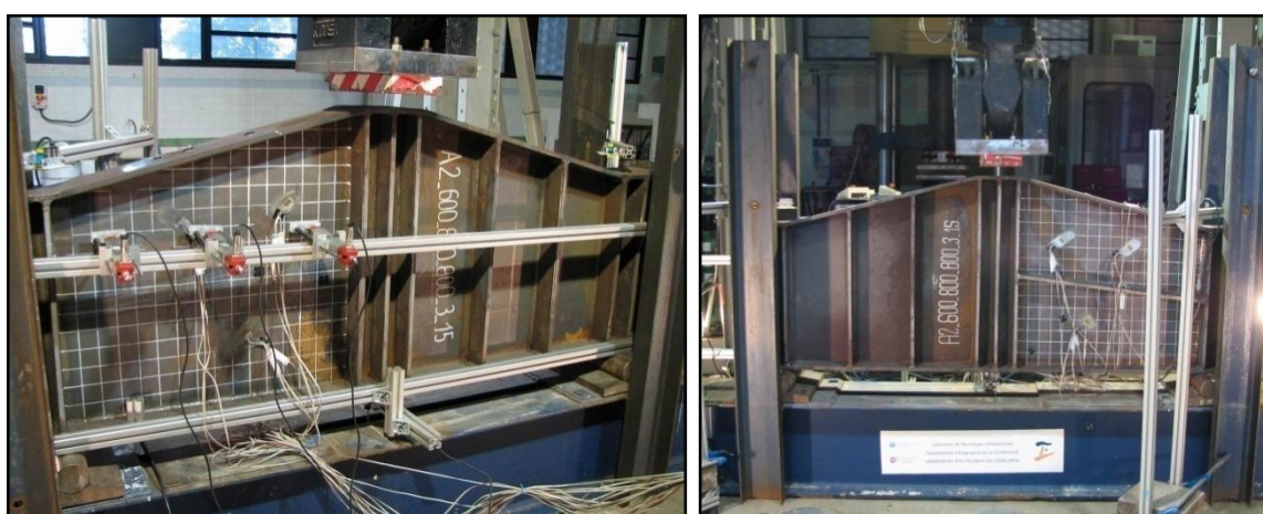
Fig. 4.2. Tested girders with the measuring equipment.
