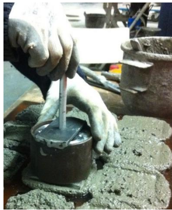
Figure 4.3.- Apparatus used to compact.
