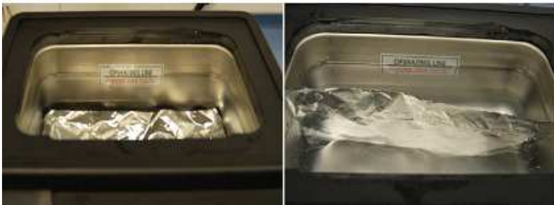
Picture 7. Placing of the aluminum sheets. Right: bottom placing. Left: Vertical placing.
