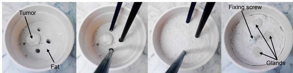
Figure 5.17: Tissue mimicking phantom manufacturing process.
