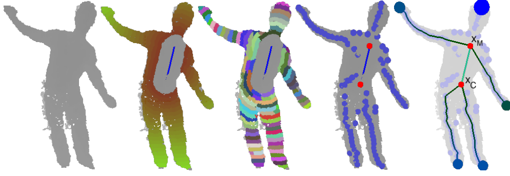
FIGURA 4.1: Summary of the steps involved in the proposed algorithm for human pose estimation. From left to right: Foreground mask, R-NBLS propagation, R-NBLS filtering, end-effector graph nodes and end-effectors found with the associated skeleton.
