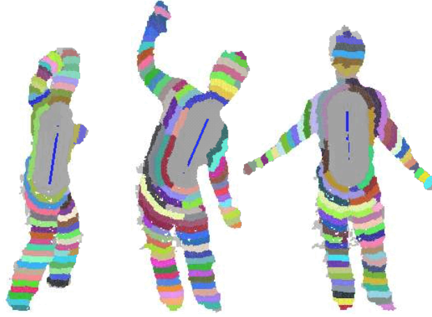
FIGURA 4.5: Three examples of narrow band filtering. The obtained regions are randomly painted. In this case, an A^{max} = 70 \text{ cm}^2 has been applied together with a (\eta_L = 30, \delta_L = 4 \text{ cm}) -connectivity.
