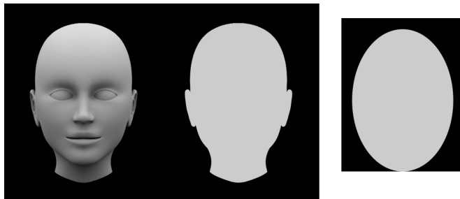
FIGURA 6.2: On the right, a graphical example of the elliptical mask \mathcal{E} used in the algorithm. On the left, a representation of a human head and its foreground mask \mathcal{F} , onto which a matching score is calculated.
