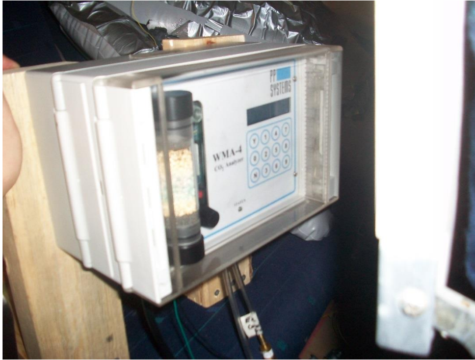
Figure 3.19 - P.P. systems CO 2 analyzer (model WMA-4)
