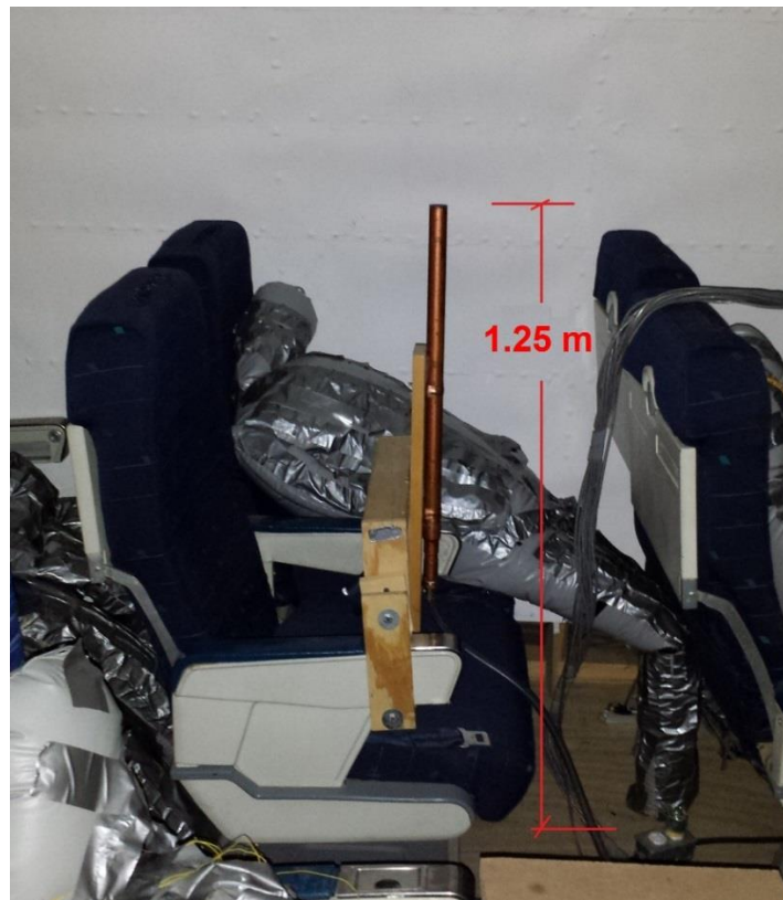
Figure 3.14 - Tracer gas injection port
