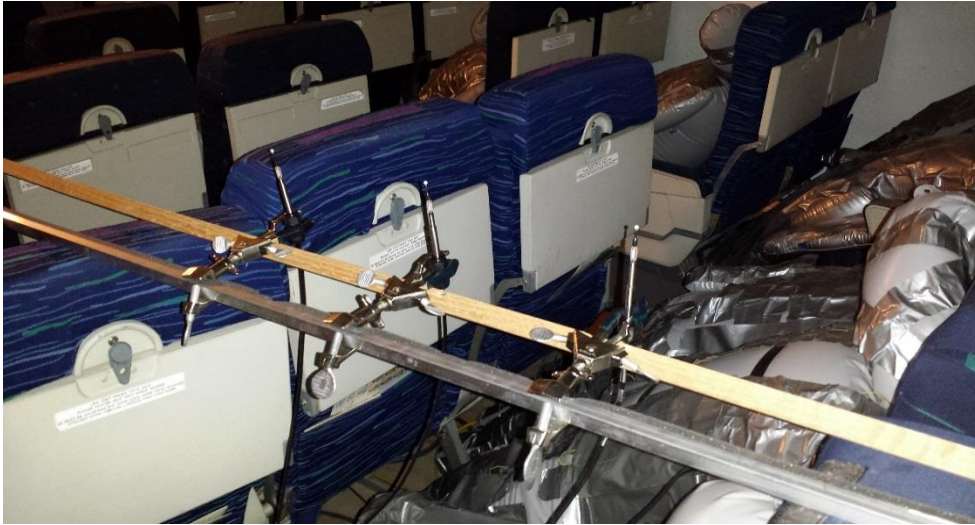
Figure 5.40 – Arrangement of the omni-directional TSI-8475 probes to investigate the separating distance between the sensors
