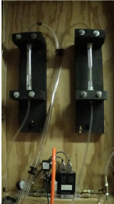
Figure 3.15 - Mass flow controllers and flow meters used to control CO 2 and Helium
