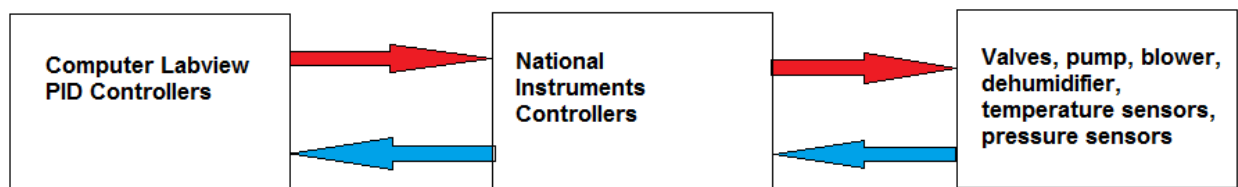
Figure 3.11 – Schematic of the supplied air control system
