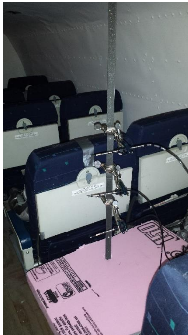
Figure G.3 – Speed transducer arrangement in the vertical direction of the cabin
