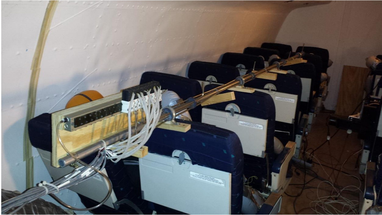
Figure 3.22 - Sampling tree showing the manifold containing the 5 solenoid valves and the exit tubing at the rear end of the manifold that was connected to the inlet of the CO 2 analyzer
