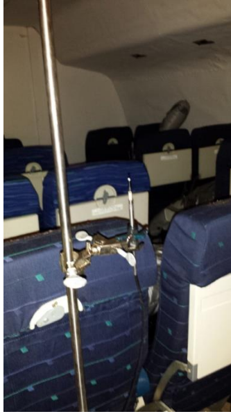
Figure 3.24 - Omni directional speed transducer used to measure airflow speed inside the mockup cabin
