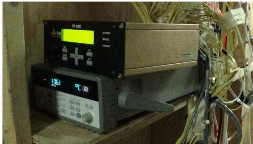
Figure 3.16 - Two channels power supply unit (top) used to control the mass flow controllers; Agilent DAQ system (bottom)
