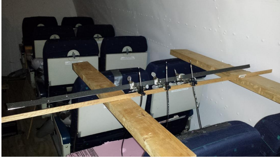
Figure G.2 – Speed transducer arrangement in the transverse direction of the cabin
