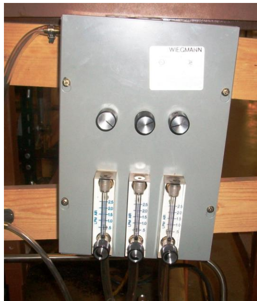
Figure 3.21 - Balance flow meters connected to the CO 2 analyzers at the inlet side and to a common vacuum pump at the exit side
