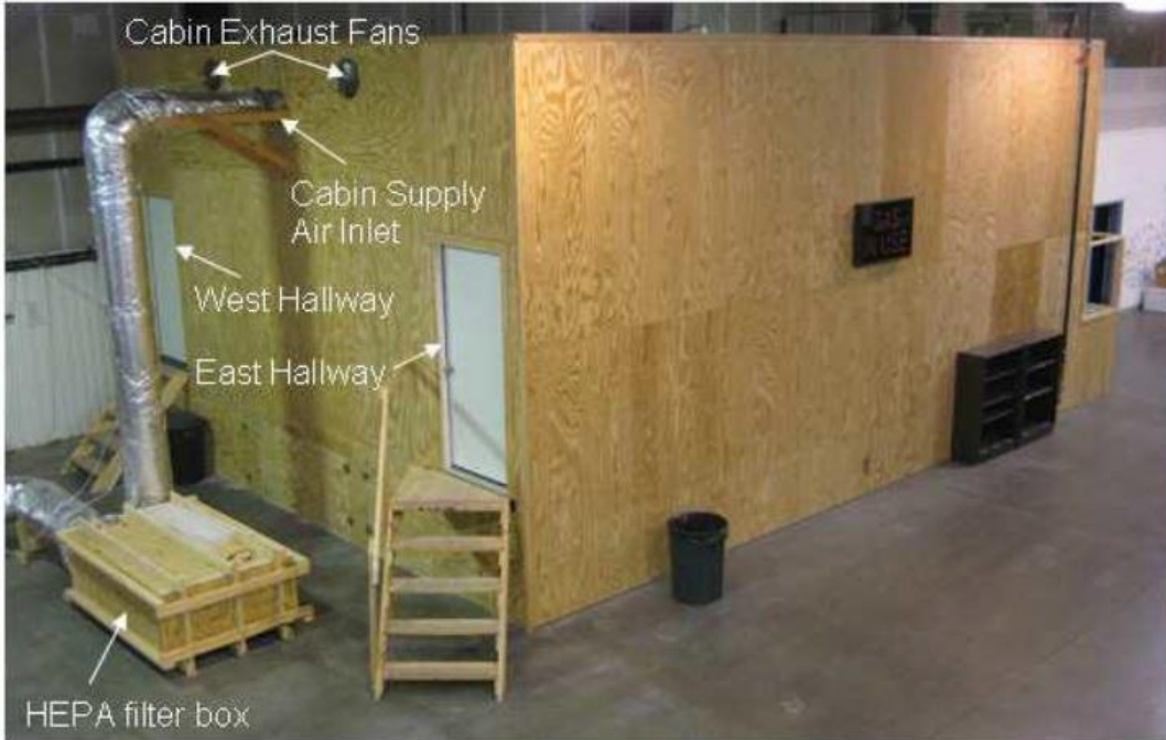
Figure 3.6 - Aircraft mockup cabin external enclosure
