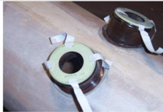
D) Close Up View of Supply Hose Connectors and Flow Restrictors
