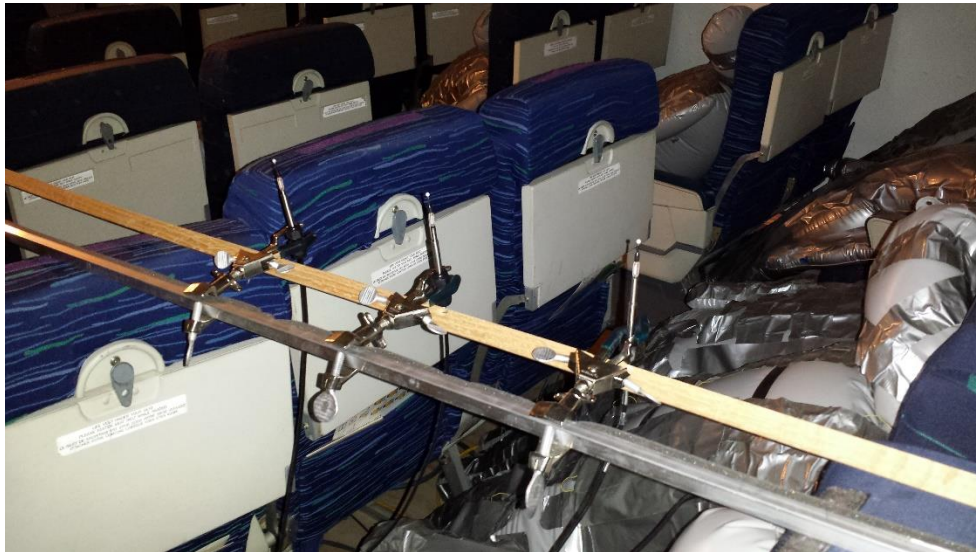
Figure G.1 – Speed transducer arrangement in the longitudinal direction of the cabin
