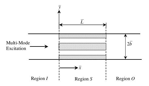
Fig. 1. (a) Plan view of silencer
