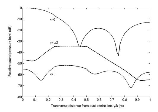
Fig. 10. Transverse sound pressure level for silencer A, at x = 0, x = L/2, and x = L, at f = 500 Hz: \_\_\_\_\_, analytic mode matching, EMED,  $(n_t = 64)$ ; \_\_\_\_\_, point collocation, EMED,  $(n_c = n_s = 65)$ .
