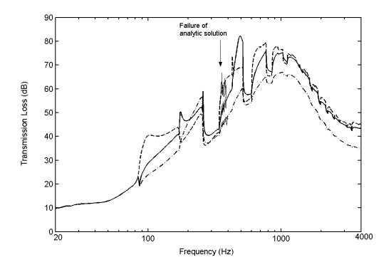
Figure 8. Predicted transmission loss for silencer C: \_\_\_\_\_, EMED; \_\_ - \_\_\_, EMA; \_\_\_\_\_, EMP. In each case, analytic solution  $(n_t = 64)$  overlays point collocation  $(n_c = n_s = 97)$ .
