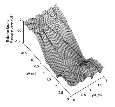
Figure 12. Sound pressure level for silencer B, EMED, at f = 516Hz ( $n_c = n_s = 65$ )
