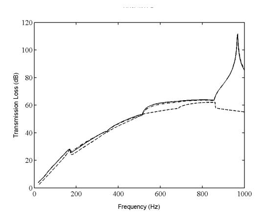
Fig. 2. Predicted transmission loss for silencer A: \_\_\_\_\_, analytic mode matching, EMED,  $(n_t = 32);$  \_\_\_\_\_, point collocation, EMED,  $(n_c = n_a = 5, n_s = 25);$  \_\_\_\_\_, point collocation, EMED,  $(n_c = n_a = 25, n_s = 125).$
