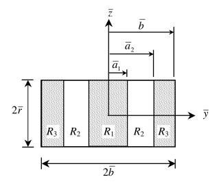
Fig. 1. (b) Silencer Cross-section
