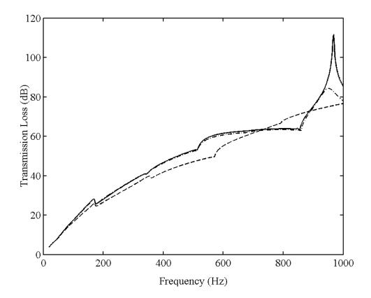
Fig. 4. Predicted transmission loss for silencer A: \_\_\_\_\_, analytic mode matching, EMED,  $(n_t = 32);$  \_\_\_\_\_, point collocation, EMED,  $(n_c = n_a = n_s = 9);$  \_\_\_\_\_, point collocation, EMED,  $(n_c = n_a = n_s = 25);$  \_\_\_\_\_, point collocation, EMED,  $(n_c = n_a = n_s = 65)$ , overlays analytic solution.
