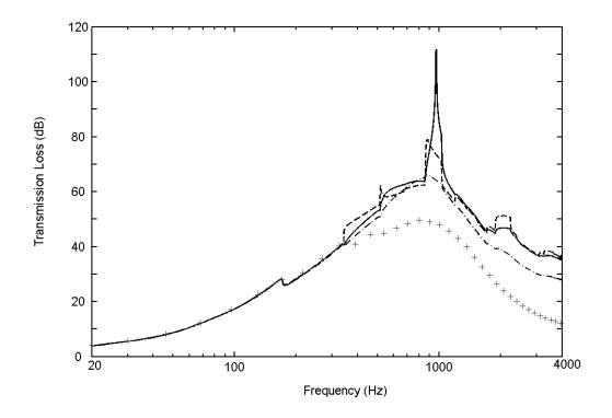
Fig. 6. Predicted transmission loss for silencer A: \_\_\_\_\_, EMED; \_\_ - \_\_\_, EMA; \_\_\_\_\_ \_\_\_\_, EMP; + , plane wave. In each case, analytic solution ( $n_t = 32$ ) overlays point collocation ( $n_c = n_s = 65$ ).
