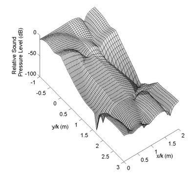
Fig. 11. Sound pressure level for silencer B, EMED, at f = 258 Hz ( $n_c = n_s = 65$ ).
