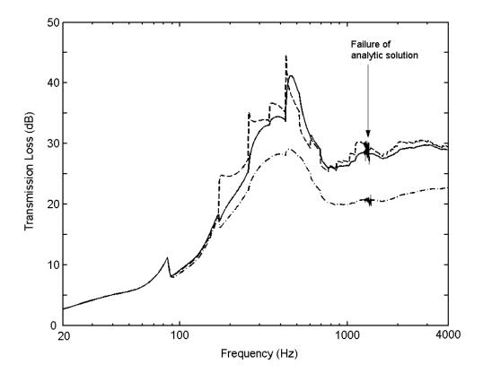
Fig. 7. Predicted transmission loss for silencer B: \_\_\_\_\_, EMED; \_\_ - \_\_\_, EMA; \_\_\_\_\_ \_\_\_\_, EMP. In each case, analytic solution  $(n_t = 64)$  overlays point collocation  $(n_c = n_s = 97)$ .
