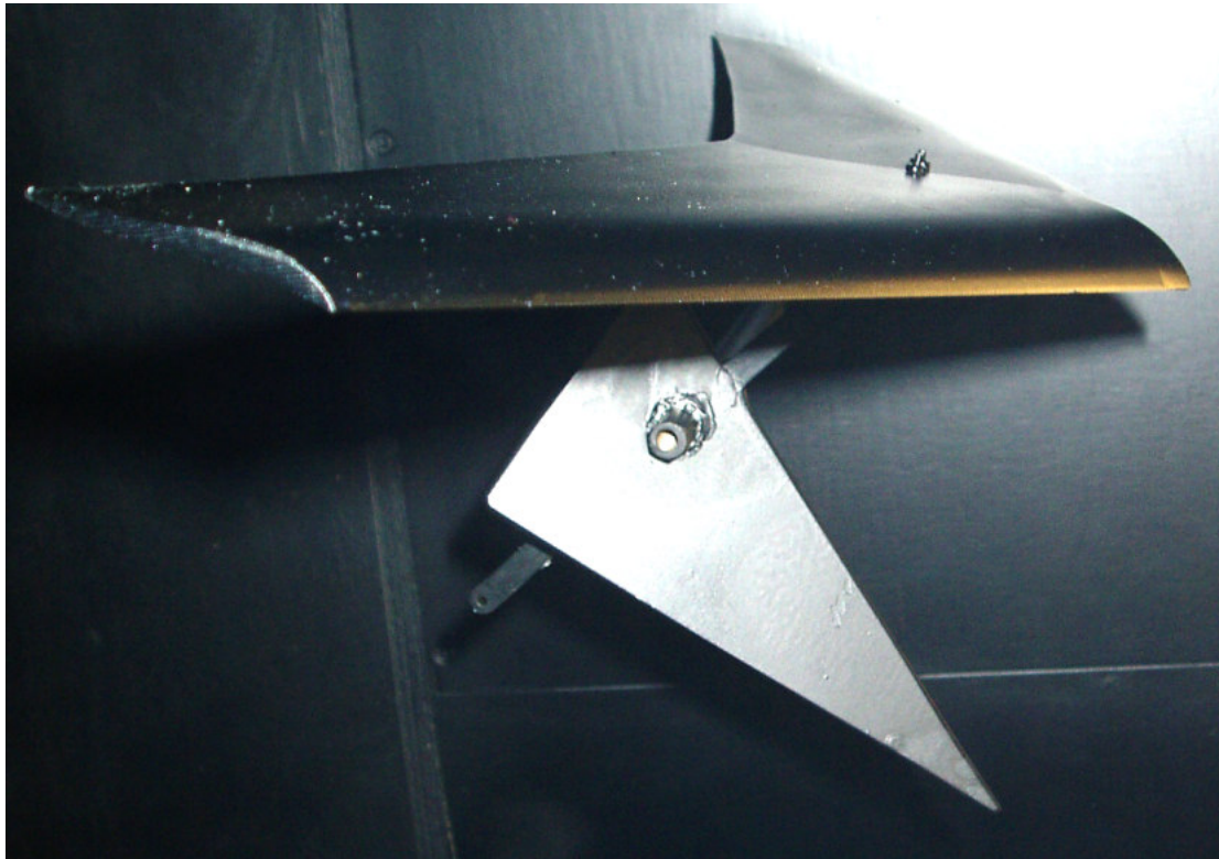
Figure 48. Scale model of Mainair Gemini Flash 2 alpha aircraft, used in wind tunnel tests
