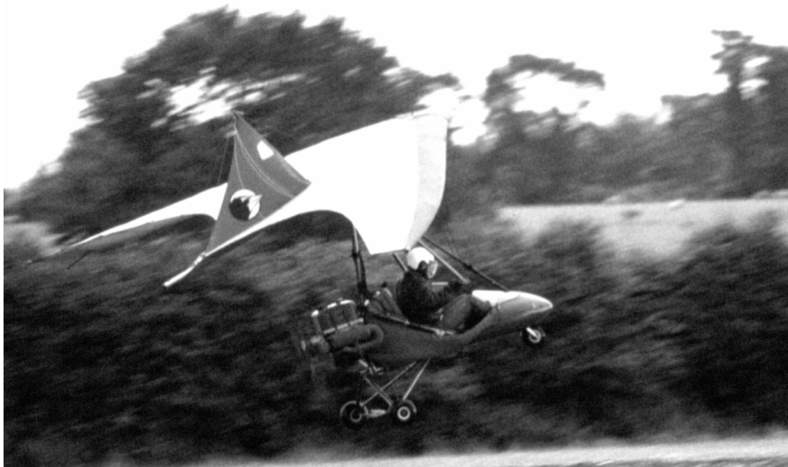
Figure 96. Southdown Raven-X with Rotax 447 engine.
