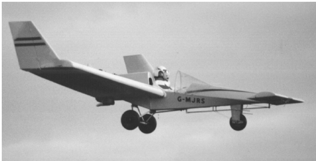
Figure 88. Eurowing Goldwing fitted with Rotax 377 engine
