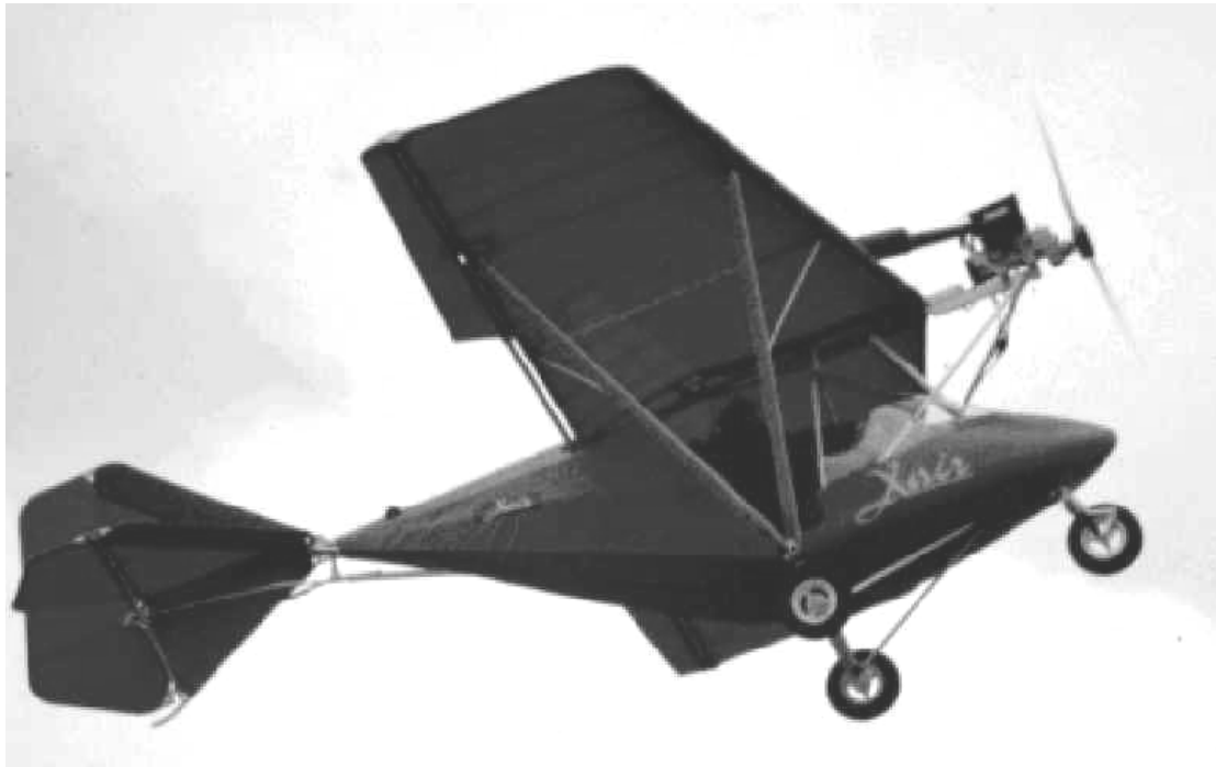
Figure 95. Raj Hamsa X'Air Mk.1 (UK) with Rotax 582/48-2V engine and Ivoprop propeller
