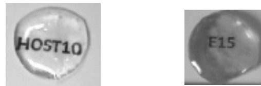
FIGURE 1. Fabricated host and \text{Er}^{3+} - \text{Yb}^{3+} doped \text{TeO}_2 - \text{ZnO} - \text{PbO} - \text{Ti}_2\text{O} - \text{Na}_2\text{O} glasses
