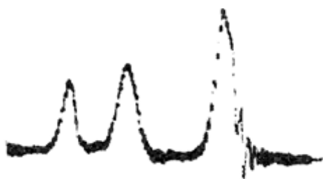
Figure 1.1: First published ^1\text{H} -NMR spectrum of EtOH. For clarity the colors of this picture were inverted. [4]
