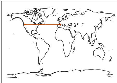
(b) Long East–West baseline. The fringe spacing ( \lambda/b ) is rather tight resulting to higher angular resolution.
