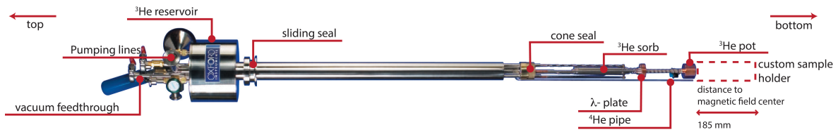
Figure 3.2: Individual components of the HELIOX VL cryostat used in a temperature range from 0.25 K to 30 K. A custom sample holder that spans the distance to the center of a magnetic field in a dewar (185 mm in the present case) can be attached to the lower end of the ^3\text{He} pot.
