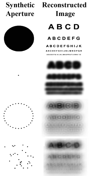
Fig. 2.5: Imaging with a completely (top) or incompletely (others) filled synthetic aperture. (Image courtesy of unknown author, and was modified).
