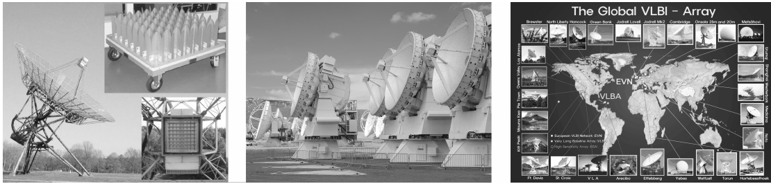
Fig. 2.4: Common radio interferometric antenna arrays and their various scales: a focal-plane array (left), a high sensitivity connected local interferometer (middle), and a network of antennas for very long baseline interferometry (right). (Images courtesy of Verheijen et al., ALMA (ESO/NAOJ/NRAO) and T.-H. Jung.)
