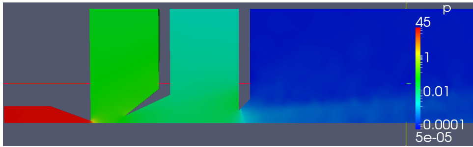
Figure 6.4 – Close up view of the simulated pressure in the upper half of the test stand close to the nozzle.
