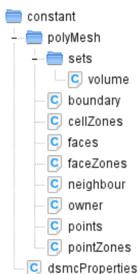
Figure 4.1 – File structure for the mesh in OpenFOAM, the structure for the full DSMC case is shown in Fig. B.1
