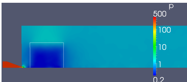
Figure 6.6 – Pressure of H atoms in state |3\rangle moving through a strong B field which is active within the region demarcated by the thin white line.
