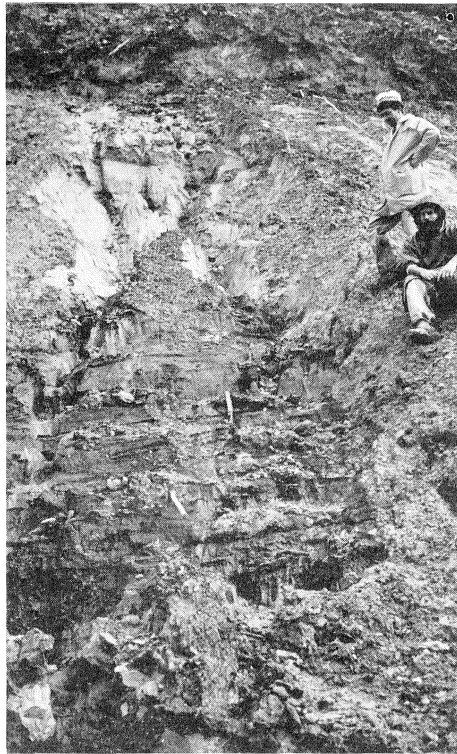
PLATE 2. Backswamp deposits at Pieman Damsite overlain by alluvial silts and slope deposits.
