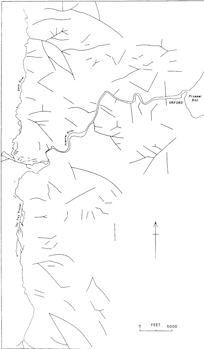
FIG 2.—Linears in the dissected area east of the Buckland Basin. The Eastern Boundary Fault is located parallel to and a short distance east of the Back and Tea Tree Rivers and is associated with strongly curved and splayed fractures.
