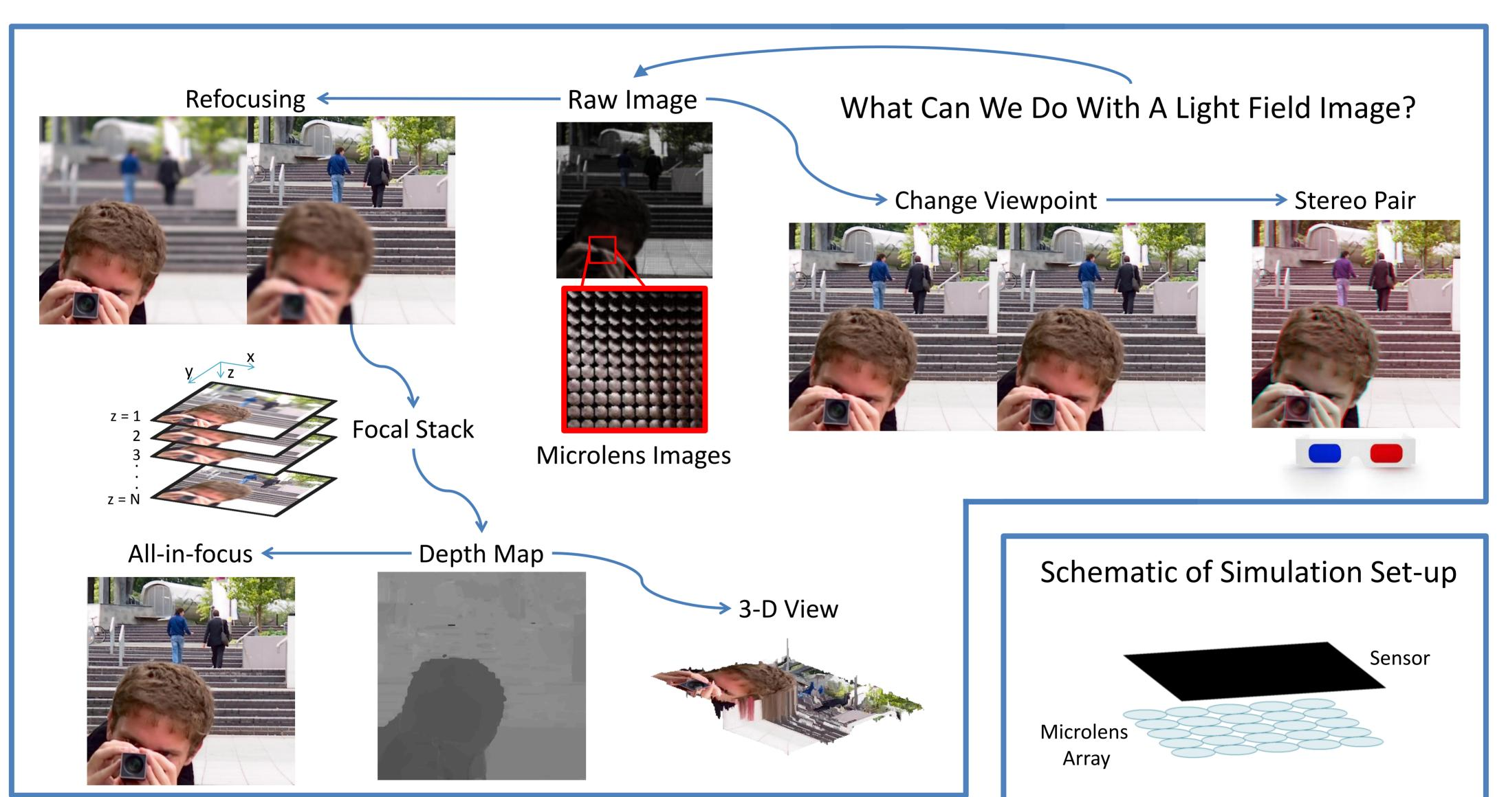
Designing, building, and optimising a light field camera can be challenging. We have created simulation and visualisation software tools to allow for virtual exploration of plenoptic cameras and data.
