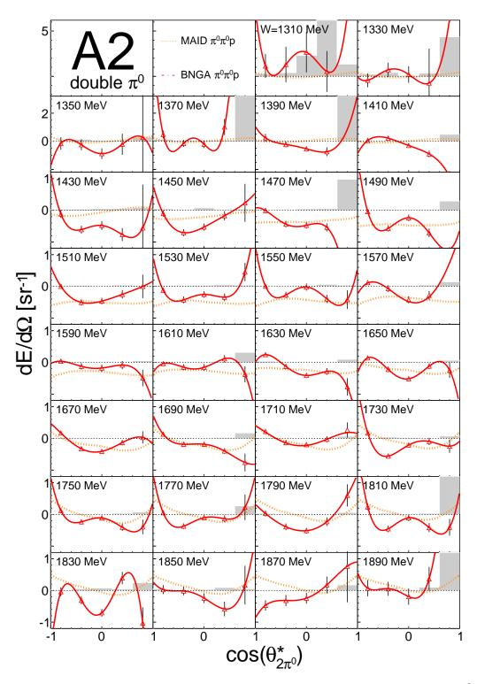
**Figure D.33:** Differential double polarization observable E for double  $\pi^0$  photoproduction from quasi-free neutrons as a function of the meson polar angle in the  $\pi^0 p$  center of mass frame. Results from the A2 data. Solid red line: Legendre fit. Dotted orange line: MAID [62]. The gray histogram at the base line of each figure represents the systematical uncertainties of the results.
