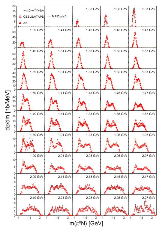
**Figure D.24:** Differential cross sections for exclusive  $2\pi^0$  photoproduction from the quasi-free neutron as a function of the  $\pi^0 n$  invariant mass. Solid red triangles: results from the A2 data. Open red triangles: results from the CBELSA/TAPS data. Dotted orange line: MAID [62].
