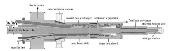
Figure 2.33: Schematic illustration of the  ${}^{3}\text{He}/{}^{4}\text{He}$  dilution refrigerator of the Frozen Spin Target used for the experiments with the deuterated butanol targets at the A2 and CBELSA/TAPS experiments at MAMI and ELSA. Figure taken from [141].
