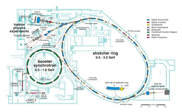
**Figure 2.16:** Floorplan of the Electron Stretcher Facility ELSA in Bonn, Germany. It shows the polarized and unpolarized electron sources with the pre-accelerator linacs (bottom left), the injector (booster) synchrotron (middle left), the storage ring (right) and the hadron physics experimental sites (top left). Figure taken from [86].
