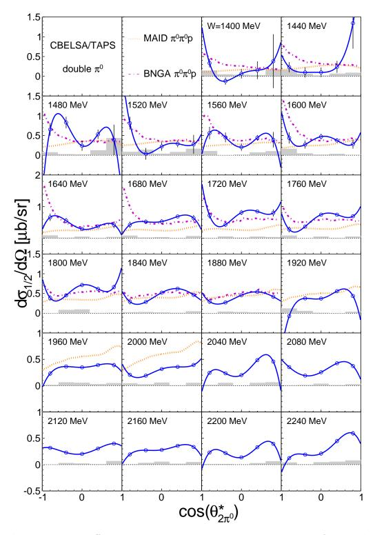
**Figure D.41:** Differential helicity dependent cross section  $\sigma_{1/2}$  for double  $\pi^0$  photoproduction from quasi-free protons as a function of the meson polar angle in the  $\pi^0 p$  center of mass frame. Results from the CBELSA/TAPS data. Solid blue line: Legendre fit. Dotted orange line: MAID [62]. Dashed-dotted magenta line: BnGa [43]. The gray histogram at the base line of each figure represents the systematical uncertainties of the results.
