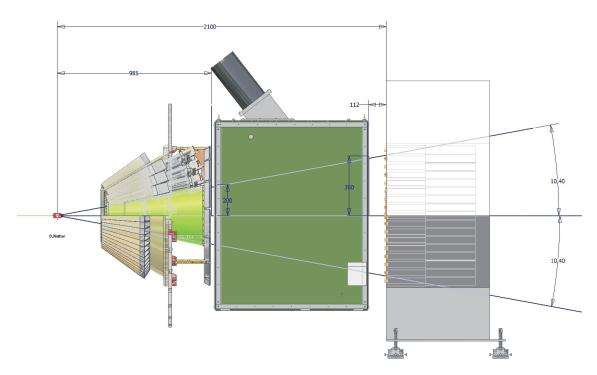
Figure 2.24: The Gas Cherenkov Detector at its place of installation between the Forward Cone Detector and the MiniTAPS Detector. Figure taken from [125].
