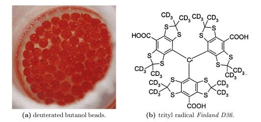
**Figure 2.32:** (a) Photograph of the deuterated butanol target material. (b) Chemical formula of the trityl radical used for the doping of the deuterated butanol target material. Photograph taken from [150], figure taken from [151].
