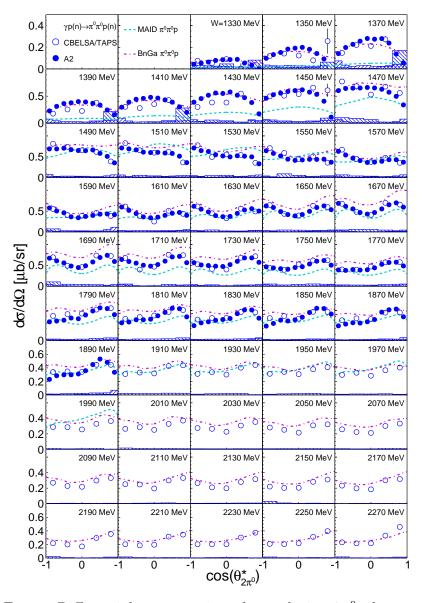
Figure D.19: Differential cross sections for exclusive  $2\pi^0$  photoproduction from the quasi-free proton as a function of the polar angle of the combined meson in the  $2\pi^0 p$  center of mass system. Solid blue circles: results from the A2 data. Open blue circles: results from the CBELSA/TAPS data. Dashed cyan line: MAID [62]. Dashed-dotted magenta line: BnGa [43]. The hatched histograms at the bottom represent the systematic uncertainty of the corresponding result.
