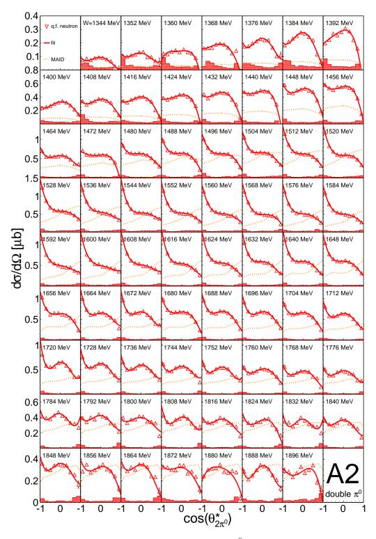
**Figure D.13:** Differential cross sections for  $2\pi^0$  photoproduction from the quasi-free neutron as function of the polar angle of the combined meson in the  $2\pi^0 n$  center of mass system. Results from the A2 data. Solid red line: Legendre fit of the data. Dotted orange line: MAID [62]. The hatched histograms represent the systematic uncertainties.
