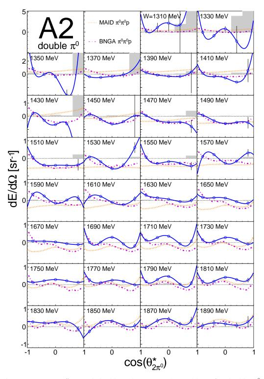
Figure D.30: Differential double polarization observable E for double  $\pi^0$  photoproduction from quasi-free protons as a function of the meson polar angle in the  $\pi^0 p$  center of mass frame. Results from the A2 data. Solid blue line: Legendre fit. Dotted orange line: MAID [62]. Dashed-dotted magenta line: BnGa [43]. The gray histogram at the base line of each figure represents the systematical uncertainties of the results.
