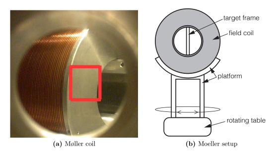
**Figure 2.30:** (a) Photograph of the Møller coil at MAMI in beam direction. (b) Schematic illustration of the Møller setup. The setup at the CBELSA/TAPS experiment at ELSA is equivalent. Photograph taken from [135], figure taken from [136].
