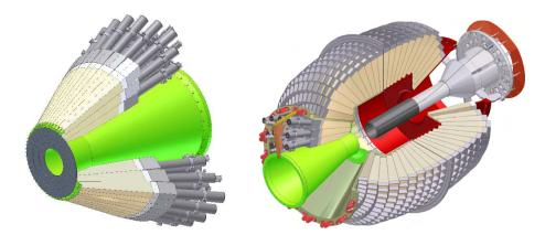
**Figure 2.21:** Schematic illustration of the Forward Cone (left) and when installed inside the Crystal Barrel detector (right). Figures taken from [118, 121].
