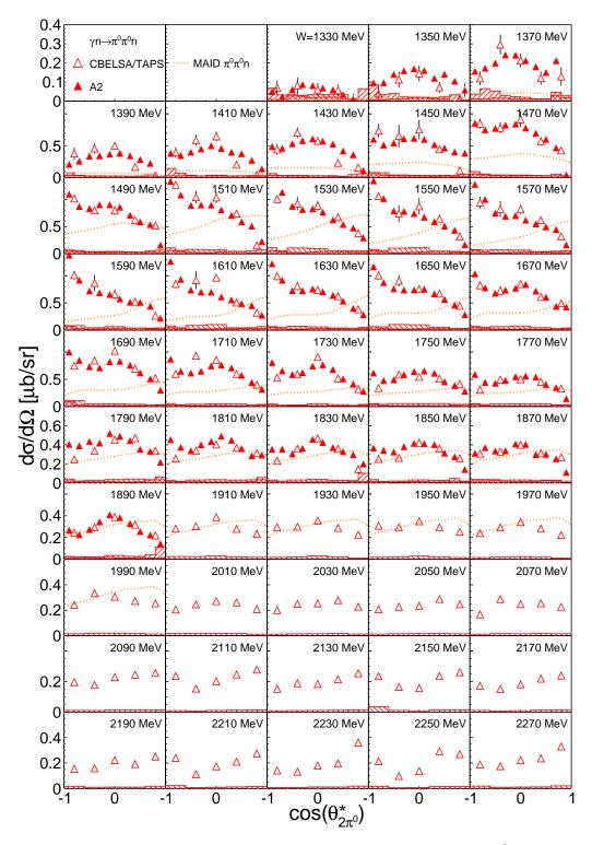
Figure D.21: Estimated differential cross sections for exclusive  $2\pi^0$  photoproduction from the free neutron as a function of the polar angle of the combined meson in the  $2\pi^0 p$  center of mass system. Solid red triangles: results from the A2 data. Open red triangles: results from the CBELSA/TAPS data. Dotted orange line: MAID [62]. The hatched histograms at the bottom represent the systematic uncertainty of the corresponding result.
