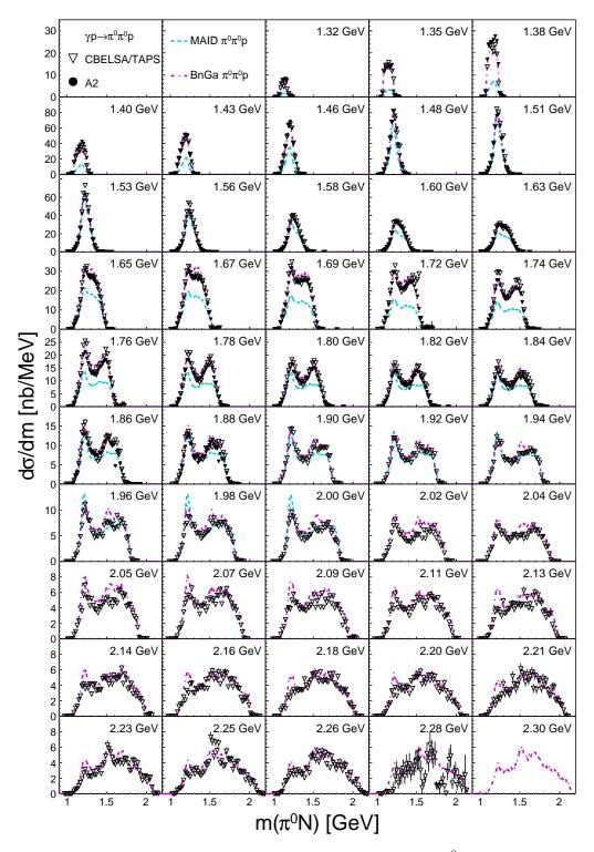
**Figure D.22:** Differential cross sections for exclusive  $2\pi^0$  photoproduction from the free proton as a function of the  $\pi^0 p$  invariant mass. Solid black triangles: results from the A2 data. Open black triangles: results from the CBELSA/TAPS data. Dashed cyan line: MAID [62]. Dashed-dotted magenta line: BnGa [43].
