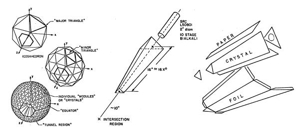
**Figure 2.9:** Schematic illustration of the Crystal Ball and its components. Left-hand side: Decomposition of the Crystal Ball geometry. Middle: Example crystal geometry. Right-hand side: Wrapping material. Figures taken from [104].
