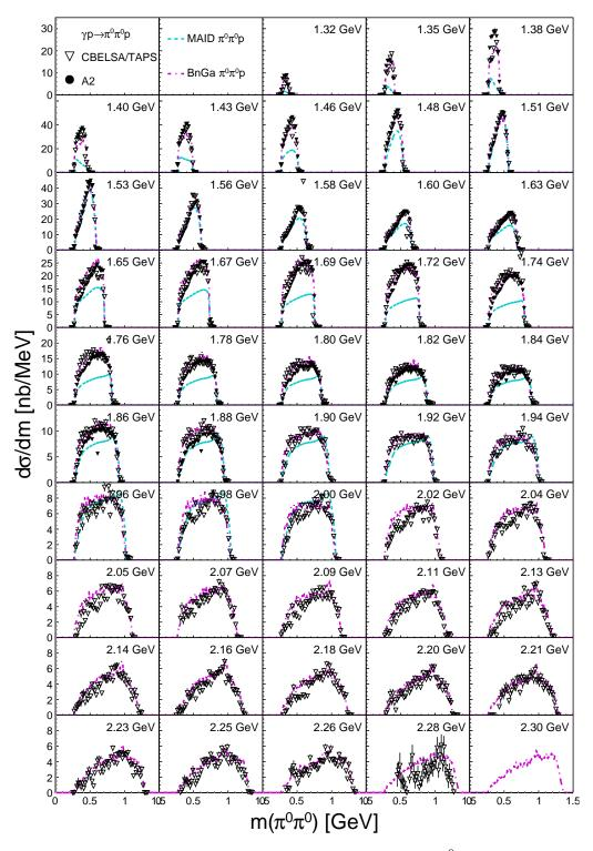
**Figure D.25:** Differential cross sections for exclusive  $2\pi^0$  photoproduction from the free proton as a function of the  $\pi^0\pi^0$  invariant mass. Solid black triangles: results from the A2 data. Open black triangles: results from the CBELSA/TAPS data. Dashed cyan line: MAID [62]. Dashed-dotted magenta line: BnGa [43].
