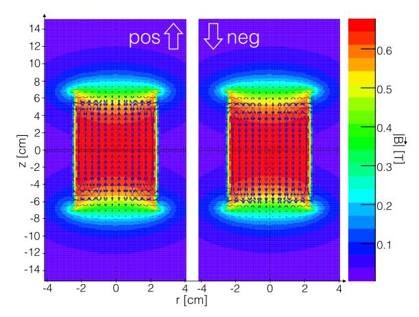
Figure 3.6: Magnetic field maps of the internal holding coil used for the simulation of A2 data with the longitudinally polarized target. Left-hand side: magnetic field in z-direction (pos). Right-hand side: magnetic field in -z-direction (neg). Size and direction of the arrows indicate the absolute value and direction of the z-component. Colors indicate the absolute value of the magnetic field.
