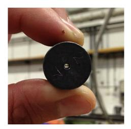
Figure 2.8: 2 mm lead collimator used for the deuterated Butanol beamtimes.
