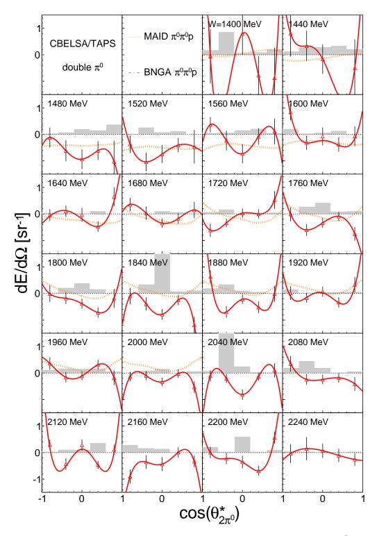
Figure D.43: Differential double polarization observable E for double  $\pi^0$  photoproduction from quasi-free neutrons as a function of the meson polar angle in the  $\pi^0 p$  center of mass frame. Results from the CBELSA/TAPS data. Solid red line: Legendre fit. Dotted orange line: MAID [62]. The gray histogram at the base line of each figure represents the systematical uncertainties of the results.
