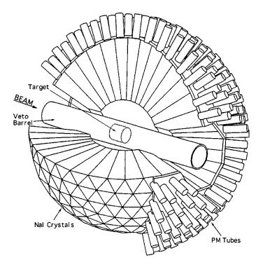
Figure 2.10: Schematic illustration of the PID (Veto Barrel) inside the Crystal Ball. Figure taken from [105].
