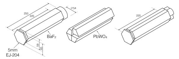
**Figure 2.12:** TAPS crystal geometries. The dimensions are given in mm. Left-hand side:  $BaF_2$  crystal with veto. Middle: Decomposition of a  $BaF_2$  crystal into four PbWO<sub>4</sub> crystals. Right-hand side: PWO<sub>4</sub> block with veto. Figure adapted from [108].
