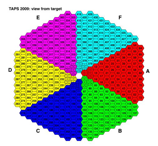
Figure 2.13: Layout and crystal numbering of the TAPS detector showing the nine outer  $BaF_2$  rings and the two inner  $PbWO_4$  rings. The six different colored sections, referred to as sectors, show the logical groups of crystals used for the trigger. Figure taken from [100].
