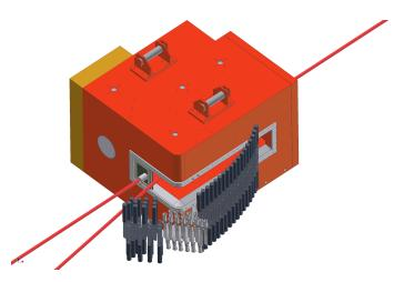
Figure 2.19: Schematic illustration of the photon tagging spectrometer at the CBELSA/TAPS experiment at ELSA. Figure taken from [116].
