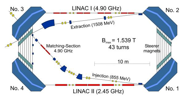
Figure 2.5: Schematic drawing of the HDSM at MAMI. Figure taken from [87].
