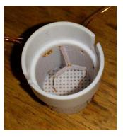
Figure 2.35: NMR coils as used for the measurement of the deuteron polarization. Left-hand side: surface coil (anti-Helmholtz configuration) used for the normal NMR measurements. Right-hand side: in-beam coil, used for the investigation of the polarization inhomogeneities of the experiments within the A2 collaboration. Photographs taken from [158].
