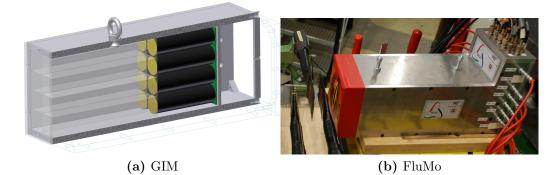
**Figure 2.25:** (a) The Gamma Intensity Monitor (GIM). (b) The Flux Monitor (FluMo). Figure taken from [118].
