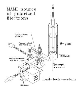
Figure 2.2: Polarized electron source at MAMI. Figure taken from [97].
