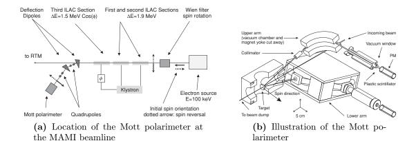
**Figure 2.29:** (a) Schematic illustration of the location of the Mott polarimeter at the A2 experiment at MAMI. (b) Schematic layout of the Mott polarimeter. The housing of the upper magnet is removed for a better visibility of the electron trajectory. Figures taken from [134].
