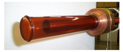
Figure 2.31: Liquid Hydrogen/Deuterium target cell used at the A2 experiment at MAMI. Photograph taken from [139].
