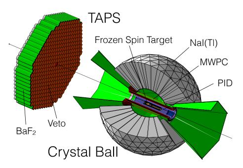
**Figure 3.2:** The A2 experimental setup at MAMI as defined in the A2 Geant4 package visualized with DAWN (Drawer for Academic WritiNgs). It shows the two main calorimeters, the Crystal Ball and TAPS and the detectors that are used to discriminate between neutral and charged particles, i.e. the Particle Identification Detector (PID), the Multi-Wire Proportional Chambers (MWPC), and the vetos. The container of the Frozen Spin Target is as well visible in the center of the Crystal Ball detector.
