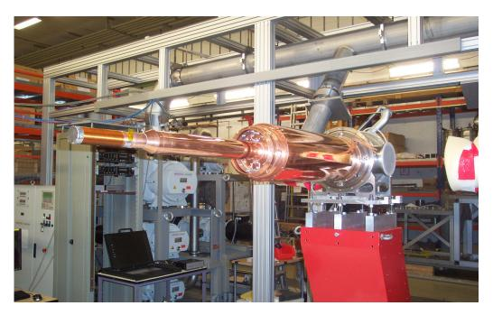
Figure 2.34: Photograph of the dilution refrigerator of the A2 experiment at MAMI. The longitudinal holding coil is mounted on its end (left-hand side of the cryostat). Photograph taken from [156].
