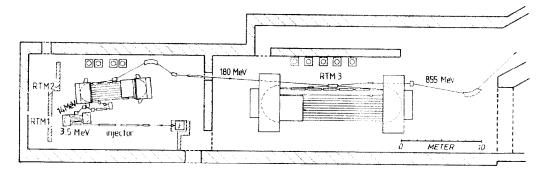
Figure 2.4: Schematic drawing of the RTM cascade at MAMI. The two first RTM stages have been used at MAMI-A and the full RTM cascade at MAMI-B. Figure taken from [98].
