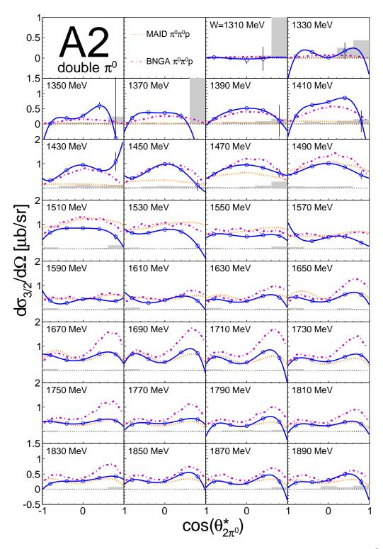
Figure D.32: Differential helicity dependent cross section  $\sigma_{3/2}$  for double  $\pi^0$  photoproduction from quasi-free protons as a function of the meson polar angle in the  $\pi^0 p$  center of mass frame. Results from the A2 data. Solid blue line: Legendre fit. Dotted orange line: MAID [62]. Dashed-dotted magenta line: BnGa [43]. The gray histogram at the base line of each figure represents the systematical uncertainties of the results.
