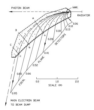
Figure 2.7: Schematic illustration of the Glasgow Photon Tagging Spectrometer. Figure taken from [102].
