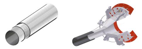
Figure 2.22: Schematic illustration of the Inner Detector (right) and of its three layers of fibers (left). Figures taken from [118].
