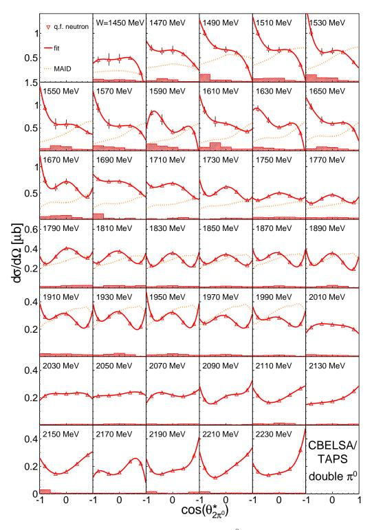
**Figure D.17:** Differential cross sections for  $2\pi^0$  photoproduction from the quasi-free neutron as function of the polar angle of the combined meson in the  $2\pi^0 n$  center of mass system. Results from the A2 data. Solid red line: Legendre fit of the data. Dotted orange line: MAID [62]. The hatched histograms represent the systematic uncertainties.
