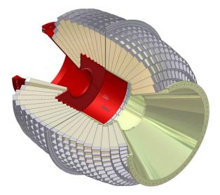
Figure 2.20: Schematic illustration of the Crystal Barrel calorimeter at the CBELSA/TAPS experiment at ELSA. Figure taken from [118].
