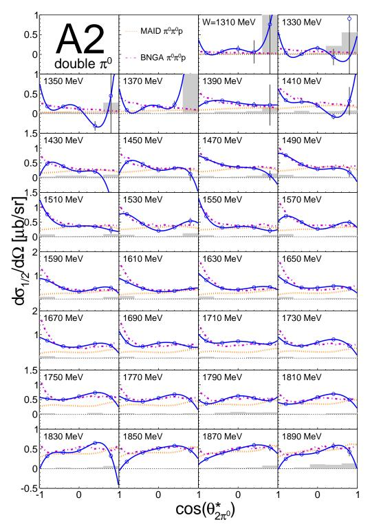
Figure D.31: Differential helicity dependent cross section  $\sigma_{1/2}$  for double  $\pi^0$  photoproduction from quasi-free protons as a function of the meson polar angle in the  $\pi^0 p$  center of mass frame. Results from the A2 data. Solid blue line: Legendre fit. Dotted orange line: MAID [62]. Dashed-dotted magenta line: BnGa [43]. The gray histogram at the base line of each figure represents the systematical uncertainties of the results.
