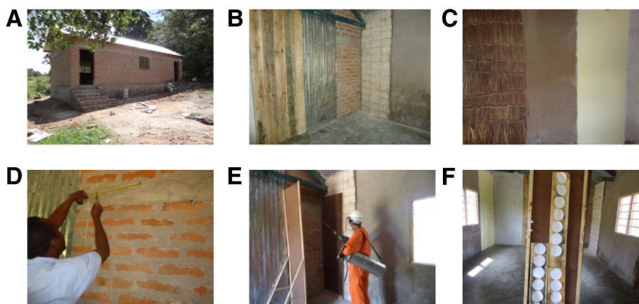
Figure 1 Design of the experimental hut and procedure used for spraying. A. An experimental hut with two rooms was constructed assembling nine different surfaces. B. Surfaces of wood, iron sheet, burnt bricks, limestone blocks and cement plastered walls are shown. C. Surfaces of palm thatch, mud daub and oil paint are shown. D. The substrates were fixed on the walls of the hut and demarcated to guide the spraying movement. E. Spraying on the tested surfaces was done using side edges to avoid overlap effect. F. Whatman paper was hinged on wood after being sprayed on tested surfaces.
