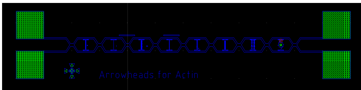
Figure 8.5: Layout of the improved device design, featuring two inlets (green, left) and two outlets (green, right) connected by two symmetric, interconnected main channels. The sorting channels are run perpendicular to the main channels (up-down).
