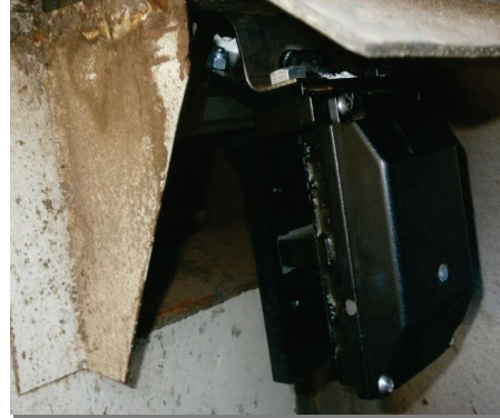
Figure 1 Shema of sensor position and picture of impact plate mass flow sensor with module behind of gape between clean grain elevator and loading auger (view from left side of grain tank)
