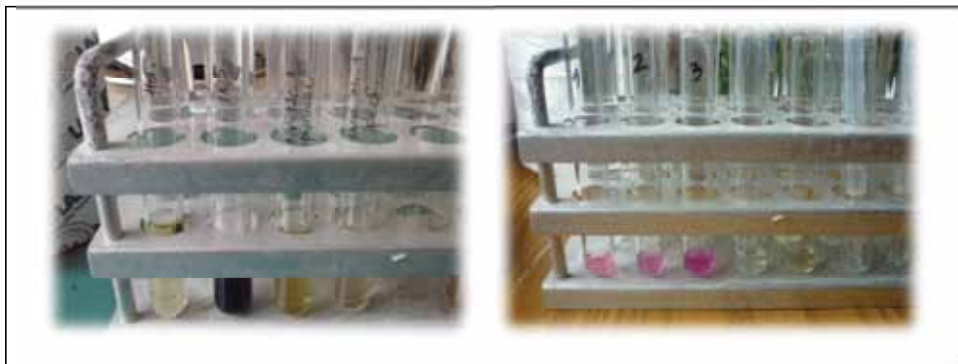
Figure 3. Micro-chemical tests for detection of starch and gelatin performed on samples from IMK Ms.1.
