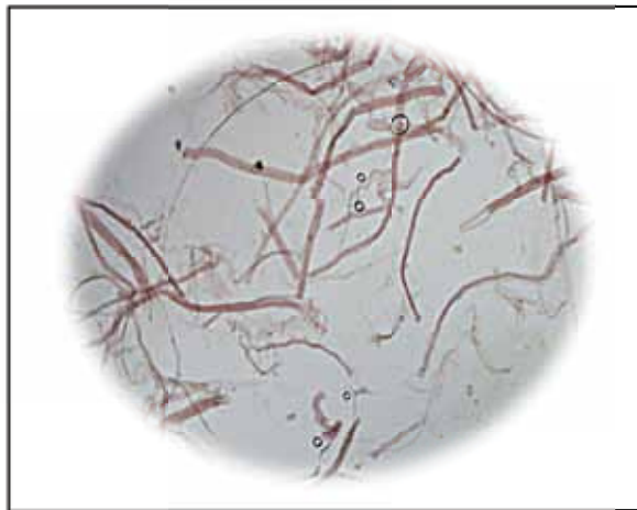
Figure 1. Microscopic view (x200) of Cotton fibers stained with Graff "C" stain.
