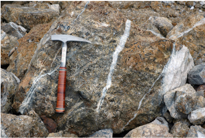
Figure 2. Pinolitic sparry magnesite with late quartz-veins of Eoalpine age from the Veitsch deposit.
