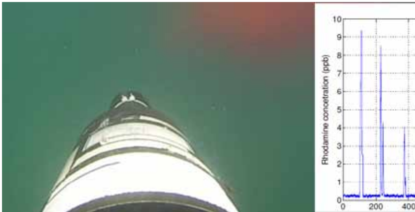
Figure 3. AUV in front of red Rhodamine plume, upper-right corner. On the right, Rhodamine concentration measurement
