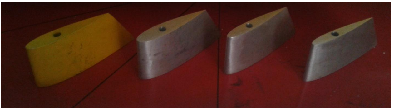
Fig.2 Four different NACA hydroplanes that installed on bare hull
