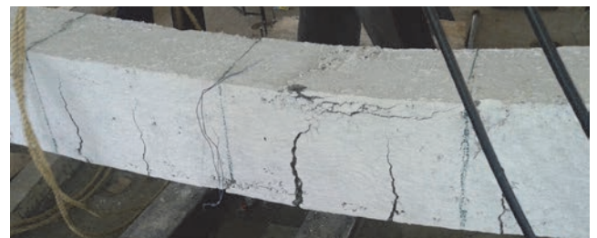
Figure 17. Crack pattern and failure mode of RC beam for copper slag 40% replacement and PP fibre 0,4%
