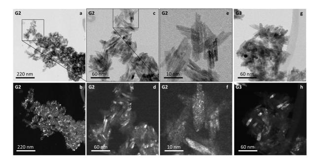
**Figure 2.** TEM images of samples G2 and G3; a, c, e and g are bright field images, b, d, f and h are the corresponding dark field images.
