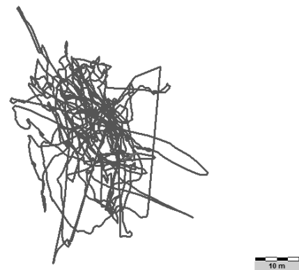
Fig. 2. Static GPS error during a 3-hour test
