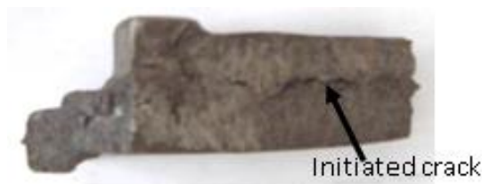
Figure 1. The as-received section of failed flywheel.
