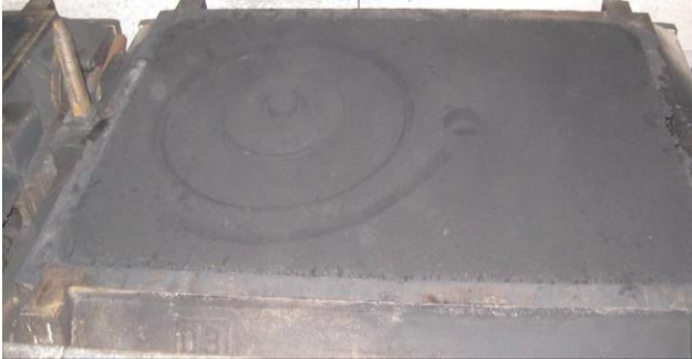
Figure 5. The upper sand mould.
