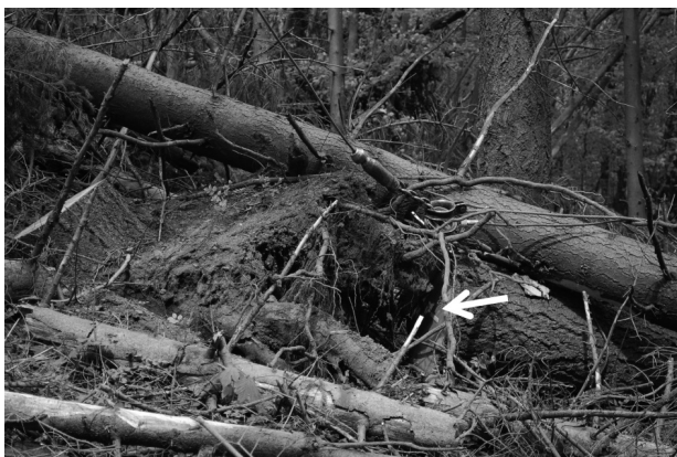
Fig. 5 Cable yarder concentration in a storm damaged forest is very challenging for the survival of tags due to the abundance of debris, deadwood and uprooted stumps, which could rip or damage the transponder (the white arrow indicates the position of the RFID tag on the log)
