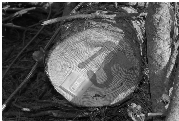
Fig. 2 Marking method with Wintag RFID and double stapling (DW)
