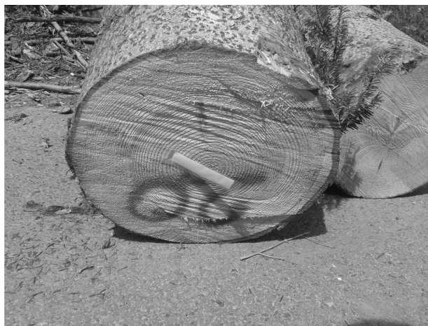
Fig. 3 Marking method with Shortdipole RFID and single stapling (SS), note the uplifted position
