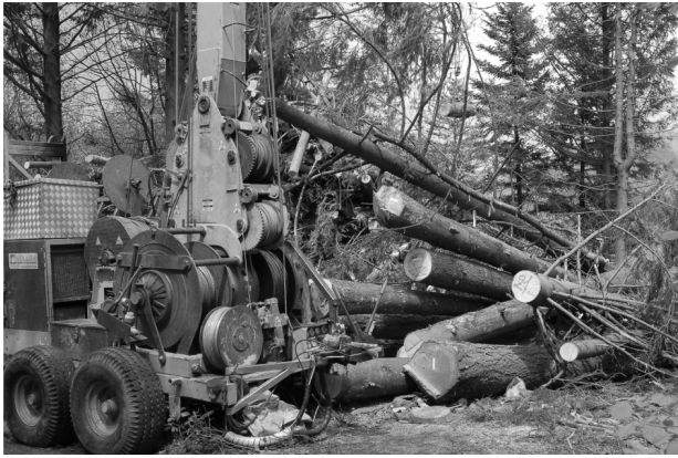
Fig. 4 Landing of cable yarder with limited operational size. In such conditions post extraction handling may cause further impacts on the tagged surfaces
