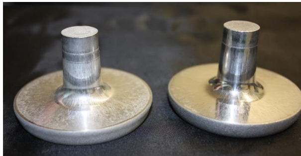
Figure 10: Surfaces of the cold impact extruded spikes: left by using lubricant 2, right with lubricant 1
