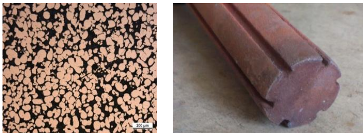
Figure 4. Sintered copper powder with grain size 50. Sintering temperature 950 °C, sintering time 30 min
