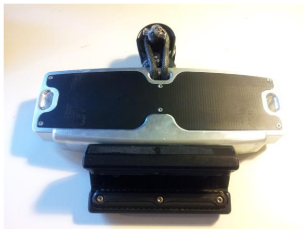
Fig. 3 Sensor element for monitoring traveller position (3DRRM)
