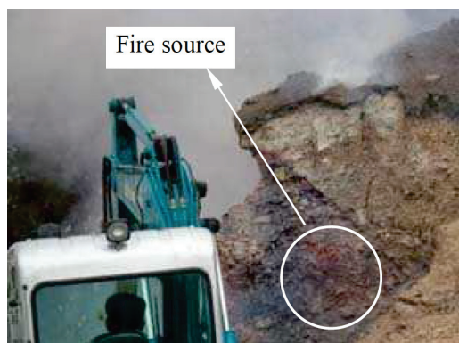
Figure 1 (a) Spontaneous combustion of millions of tons of ores at an ore field in Guizhou Province
