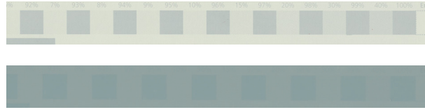
Figure 1: Contrast between exposed and not exposed areas on a processed plate (top) and on a not processed plate (bottom)
