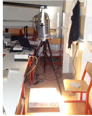
Figure 2 Experimental setup of the thermal excitation, heating distance of 1.5 m from the specimen surface
