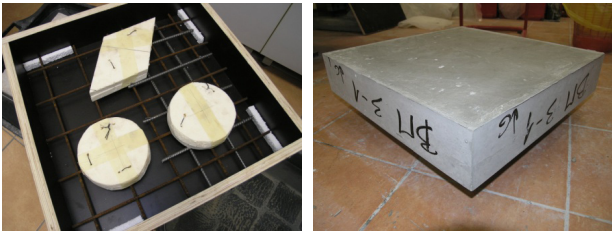
Figure 4 Concrete test specimen with polystyrene defects, preparation stage and finished specimen
