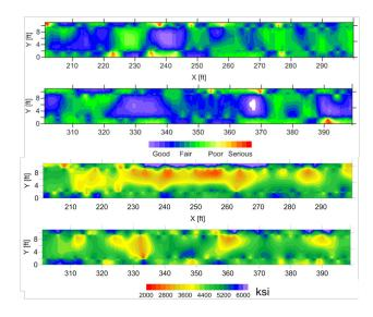
*Figure 6* Delamination map (top) and concrete modulus map (bottom).
