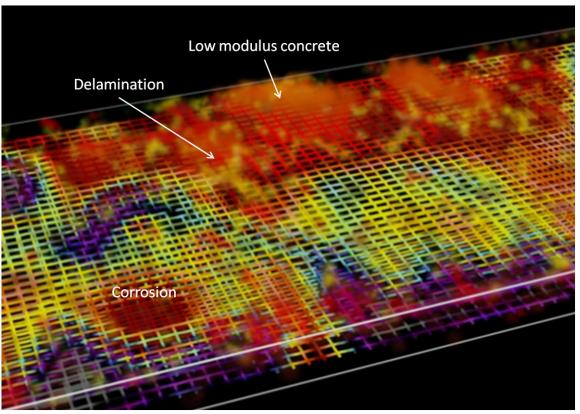
*Figure 8* 3D visualization of the detected deterioration and defects.
