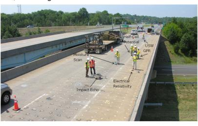
**Figure 2** Most commonly used NDE technologies in detection of corrosion induced deterioration.
