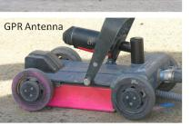
*Figure 3* Samples of probes and devices of NDE technologies implemented in RABIT.
