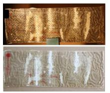
Figure 15 Impacted and severely delaminated specimen
