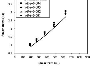
Fig. 6 - Shear stress versus shear rate; nano-fluids are showing the Newtonian behavior
