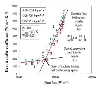
Fig. 10 – Influence of heat and mass flux on convective boiling heat transfer coefficients
