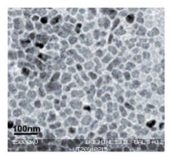
Fig. 2c - TEM image of CuO (II) nanoparticles
