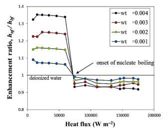
Fig. 12 – Influence of concentration on convective boiling heat transfer coefficient of CuO/water nano-fluid (G=353 kg m<sup>-2</sup> s<sup>-1</sup> and sub-cooling level = 313 K)
