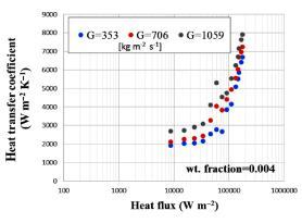
(e) Flow boiling heat transfer coefficient of CuO/water; wt. fraction: 0.004 Fig. 11 – Influence of heat and mass flux on flow boiling heat transfer coefficient of CuO/water nano-fluid
