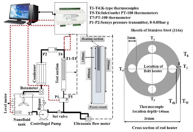
Fig. 1 – Scheme of test loop
