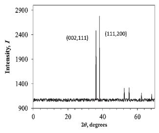
Fig. 2a - XRD pattern of CuO (II) nanoparticles
