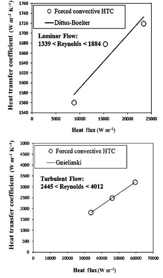
Fig. 9 – Experimental results for deionized water in laminar and turbulent flow in comparison with well-known correlations
