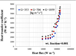
(b) Flow boiling heat transfer coefficient of CuO/water; wt. fraction: 0.001
