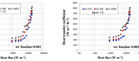
(c) Flow boiling heat transfer coefficient of CuO/water; wt. fraction: 0.002
