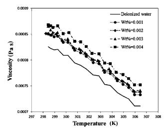
Fig. 8 – Viscosity of CuO/water nano-fluid at different temperatures
