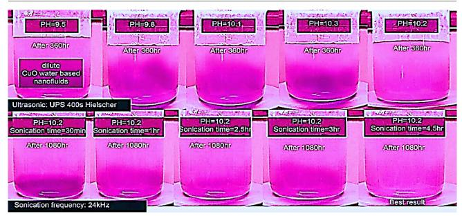
Fig. 3 - Stability of CuO nano-fluid using pH control, stirring and sonication process
