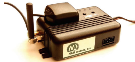
Figure 2 ONI System on-board unit Source: authors
