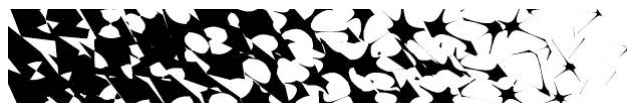
Figure 5 Controlled stochastic dispersing of the screen for tones lower than 50 % surface coverage with Postscript interpretation
