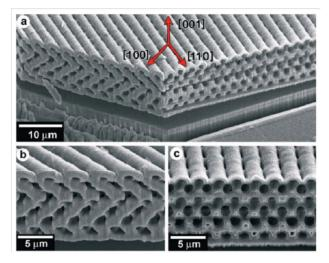
**Figure 8.** Scanning electron microscopy views of a germanium photonic crystal with a diamond-based woodpile structure. The sample was fabricated by the direct ink writing of a template followed by chemical vapour deposition of germanium. This structure has a complete photonic band gap in the infrared region of the electromagnetic spectrum. Adapted from reference [24]. Copyright Wiley-VCH Verlag GmbH & Co. KGaA. Reproduced with permission.
