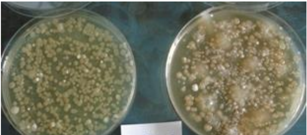
Figure 4: Mixed microbial culture isolated on two different growth media (TSA, MEA) from laboratory vessel bottom with euro diesel after 3 month of storage
