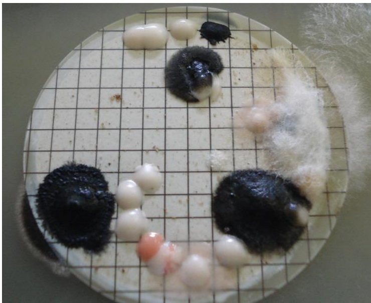
Figure 2: Mixed microbial culture isolated on MEA from the bottom of laboratory FAME tank after 2 month of storage
