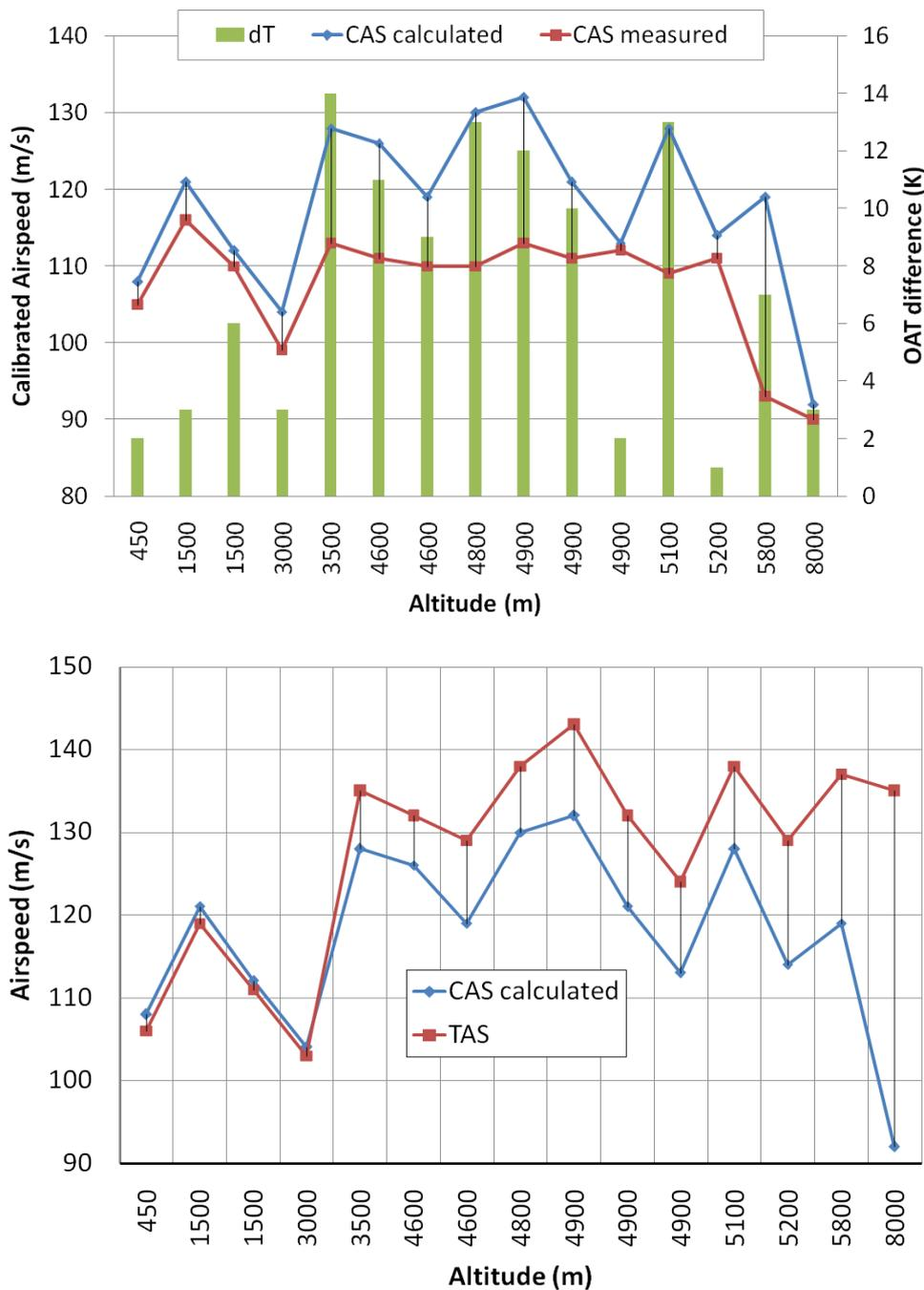
Fig. 3 Variation in CAS, TAS, and OAT with flight altitude. Plots were generated from the data in Tables 1-2
