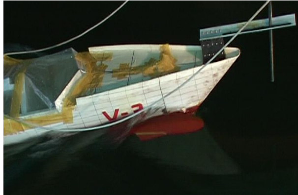
Fig.17 Picture of seakeeping performance in irregular waves of hybrid monohull
