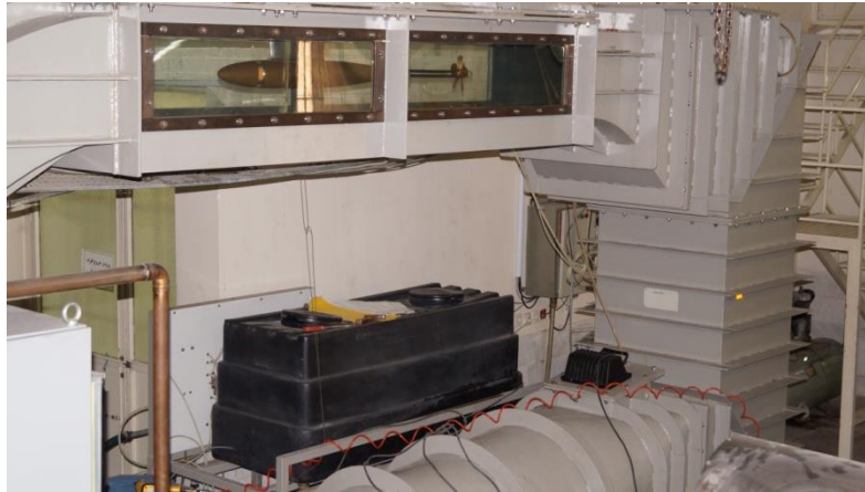
Fig. 3 Test section K23 cavitation tunnel
