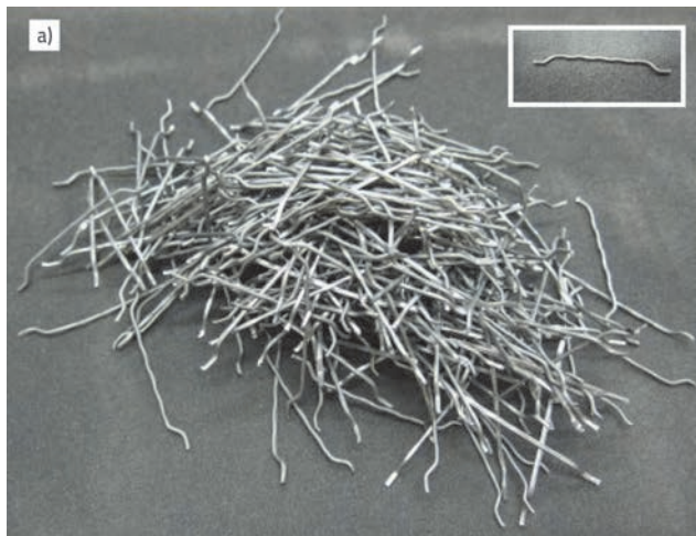
Figure 1. Materials used: a) Steel fibres; b) PP fibres
