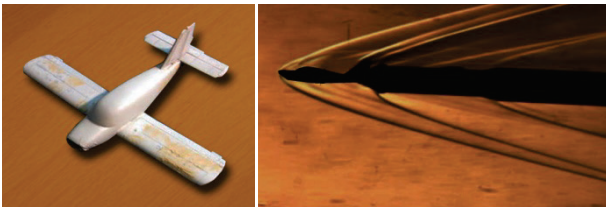
Figure 8 3D printed airplane and tested airplane in a wind tunnel
